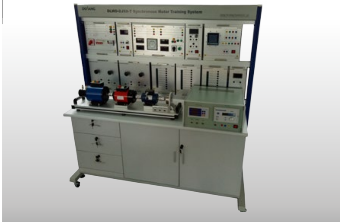
DLWD-DJSX-T Synchronous Motor Training System
